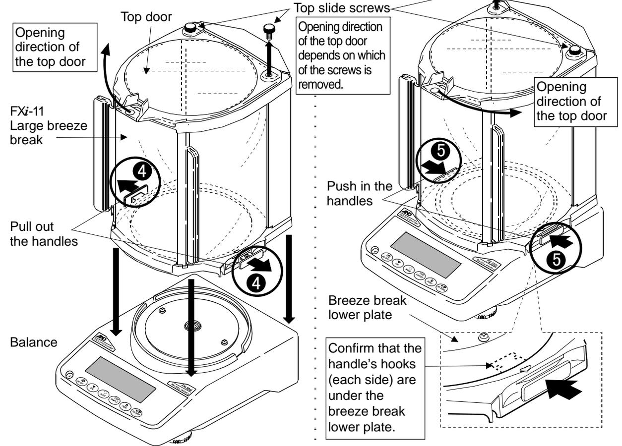
6. Install the pan support on the pan support boss and install the weighing pan on the pan support.
