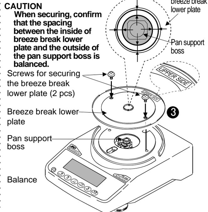
**CAUTION** - When installing, use care not to apply excessive load to the sensor mechanism (circumference of the pan support boss) of the balance.
