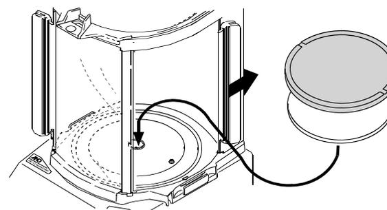
**CAUTION** - When transporting the balance, do not hold the breeze break. Hold the balance.
