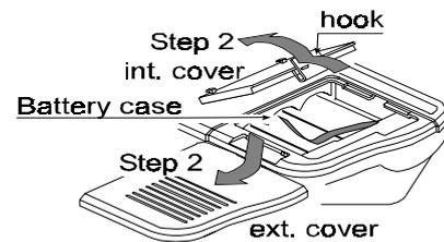
Step 3 Insert six new dry cells ensuring correct polarity (+,-). Battery size is 'D'
