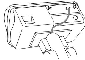
Step 2 Press and slide to open the external cover. Press the hook of the internal cover to the left side and lift the cover.
